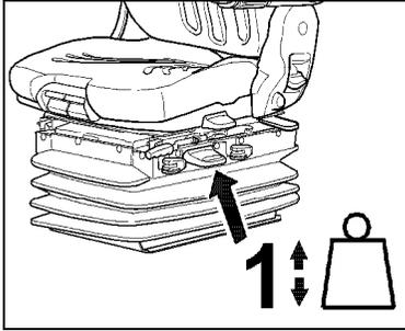
The seat must be adjusted for the driver's weight by briefly pulling the actuator lever of the automatic weight and height adjuster (arrow) with the vehicle at a standstill and the driver sitting on the seat.
