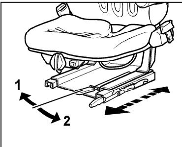
Under certain driving conditions (for example with a trailer attached), it is useful to activate the fore/aft isolator. This means that shock impacts in the driving direction can be better absorbed by the driver seat.
