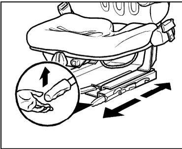
The fore/aft adjustment is released by lifting the locking lever.
